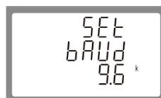
From the set-up menu, use buttons **2** and **3** to select the Baud Rate option.
