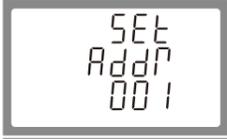
From the set-up menu, buttons **2** and **3** to select the address ID.
