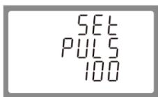
From the set-up menu, use buttons **2** and **3** to select the Pulse width option.
