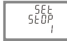
From the set-up menu, use buttons **2** and **3** to select the stop bit option.
