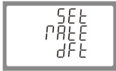
From the set-up menu, use buttons **2** and **3** to select the Pulse Rate option.
