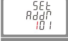
Press button **4** to enter the selection routine. The current setting will be flashing.
